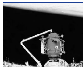
Figure 11-5 Canadarm being used to install the shuttle docking port on Mir.
